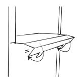
Also fold C along the folding lines on the front and click the fingers into base part A.
