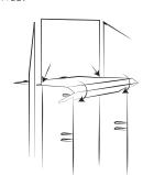
Fasten upper shelf C in the window of base part A and fold C to fit into the incisions of legs B.
