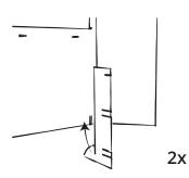
3. Slide the legs B in the insicions at the bottom of A. Do this on both sides.
