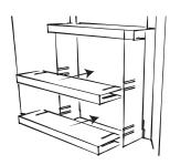
Fold back shelf along the folding lines and slide into the incisions of the legs. Do this for both shelfs.
